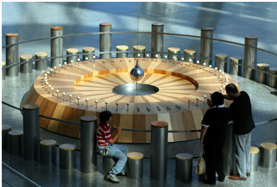
Figure 4.4 Foucault's Pendulum. As Earth turns, the plane of oscillation of the Foucault pendulum shifts gradually so that over the course of 12 hours, all the targets in the circle at the edge of the wooden platform are knocked over in sequence. (credit: Manuel M. Vicente)
